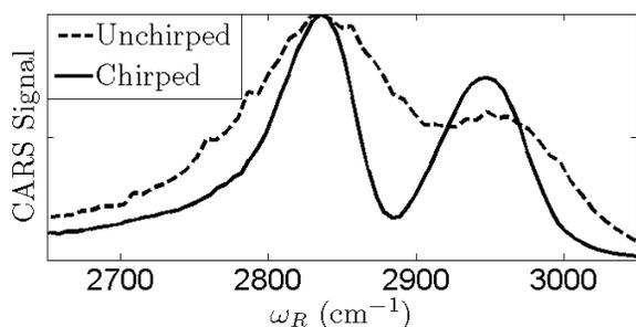
**Figure 2:** CARS spectra of methanol obtained by scanning the time delay between the pump and Stokes pulses shown in Fig. 1. The dashed curve was for unchirped pulses, the solid for which pulses width matched chirp rates.
