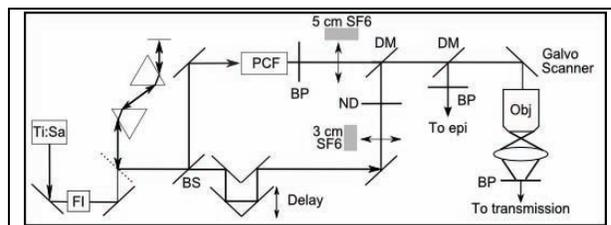
**Figure :** Simple CARS Microscope. A 50:50 beam splitter (BS) splits pulses from an isolated (FI), prism compressed Ti:Sa oscillator. One half went to a PCF and bandpass filter (BP) before being recombined on a dichroic mirror (DM). The other half was time delayed and attenuated (ND). Glass blocks (SF6) controlled the chirp rates. The recombined pulses were sent into the FV300 microscope for imaging.
