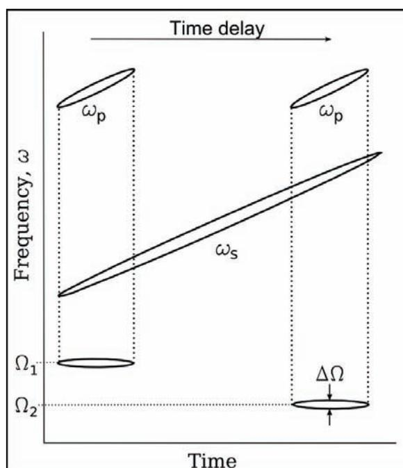
**Figure 1:** Time-frequency plots of chirped Pump and Stokes pulses. The CARS spectral resolution  $\Delta\Omega$  is determined by the height of the difference frequency ellipse  $\omega_p - \omega_s$ . Adjusting the chirp rates gives an adjustable instantaneous bandwidth and a user-variable spectral resolution. Changing the time delay of the Pump relative to the broadband Stokes scans this instantaneous difference frequency, probing different Raman modes ( $\Omega_1, \Omega_2$ ).
