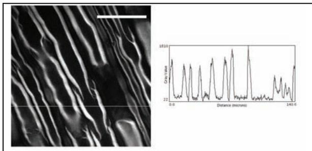
**Figure 4:** Forward detected FV300 CARS imaging of fixed rat dorsal root nerves at  $2850\text{ cm}^{-1}$  (lipid C-H stretch). The lipid-rich myelin sheath surrounds the neuronal axon and generates a strong CARS signal. The pixel intensity profile of the indicated line is shown, revealing high contrast. The scale bar is  $50\text{ }\mu\text{m}$ . The pixel dwell time was  $8\text{ }\mu\text{s}$ . [3]
