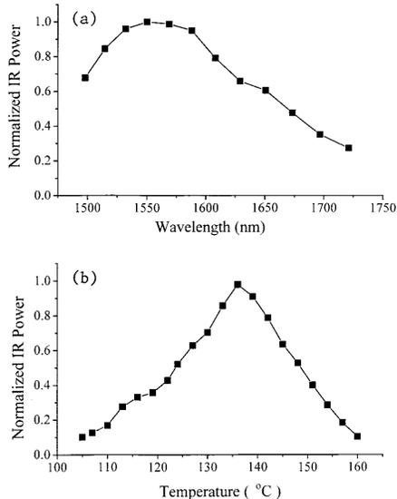
Fig. 2. (a) Wavelength tuning curve of LBO crystal for generation of 1.588- $\mu\text{m}$  femtosecond pulses at  $T = 135^\circ\text{C}$ . (b) Temperature tuning curve of LBO crystal for generation of 1.588- $\mu\text{m}$  femtosecond pulses.
