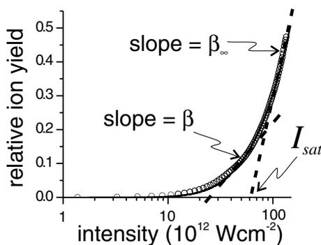
FIG. 1. A typical intensity scan, shown here for the Nb atom. The ion yield is plotted vs the logarithm of the peak intensity. A multiexponential fit to the data is shown as a solid line. The limiting slope  $\beta_{\infty}$ , its intercept  $I_{\text{sat}}$ , and the slope  $\beta$  at a lower intensity are shown. As discussed in the text,  $\beta$  was used to extract the absolute ionization rates. All other atoms (not shown) were treated in a similar manner.
