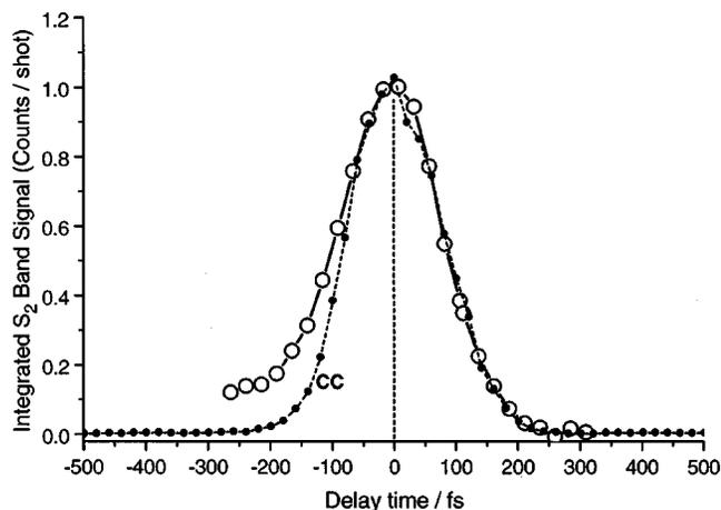
FIG. 7. Energy integration of the peak at  $\epsilon_1 = 2.3$  eV shown in Fig. 6(b), plotted as a function of time. It can be seen that, for positive times, this signal follows the cross-correlation signal (CC, dashed line) indicating that the internal conversion time scale is much less than 100 fs. For negative time delays, the excited state dynamics of a higher lying state can be seen. For a discussion, see the text.
