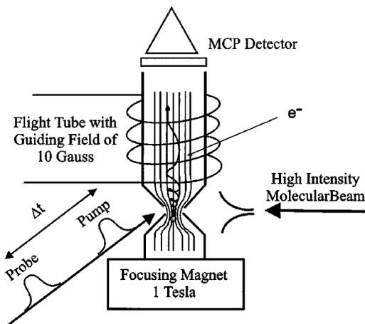
FIG. 1. Schematic sketch of the magnetic bottle photoelectron spectrometer. A skimmed molecular beam enters the interaction region of the magnetic bottle. The strongly divergent 1 T magnetic field parallelizes electron trajectories in the upper-half plane. These are guided in a 10 G field toward a detector. In a typical experiment, photoelectron kinetic energy spectra are recorded as a function of time delay.
