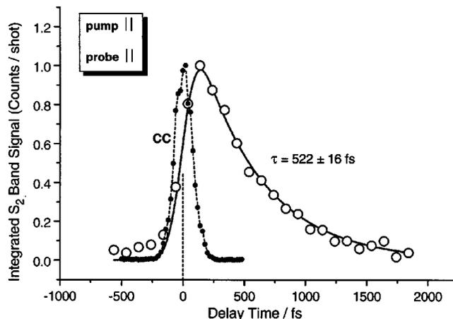
FIG. 3. Energy integration of the peak at  $\epsilon_1 = 2.5$  eV shown in Fig. 2(b), plotted as a function of time. The solid line is a fit to a convolution of a monoexponential decay of time constant  $522 \pm 16$  fs with a Gaussian cross-correlation function (CC, dashed line) of width 170 fs FWHM. This determines the  $S_2$  lifetime to be  $522 \pm 16$  fs.
