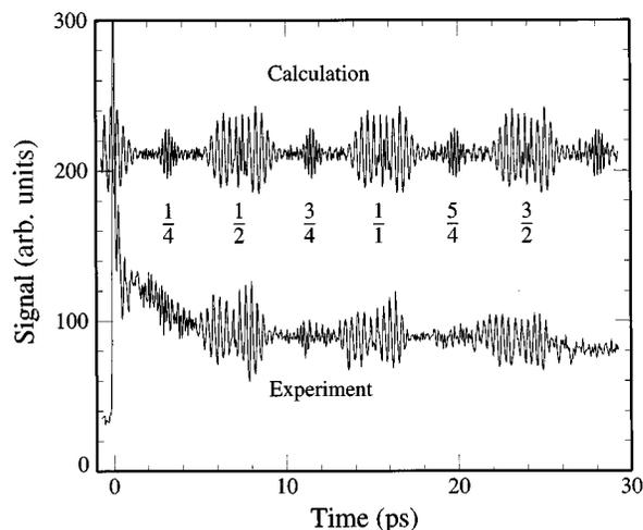
FIG. 1. Pump-probe scan showing Br<sub>2</sub><sup>+</sup> as a function of time delay, with a pump wavelength of 560 nm and a probe wavelength of 290 nm. Bottom trace is experimentally measured, upper trace is calculated. The signal is a measure of when the wave packet is near its inner turning point. Higher-frequency components are due to fractional revivals of the wave packet, as indicated by the assignment ( $p/q = \frac{1}{4}, \frac{1}{2}, \dots$ ).
